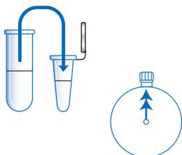
The red color should slowly fade to a rose color, then to orange, and finally, when the reaction is complete, completely to yellow. Try to be accurate in timing reaction. One variable may be your judgment of when the reaction is yellow. At this point, note the time again or stop the timer and record.
